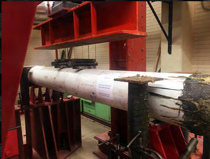
Four Point Test set up at the University Structural Lab.
