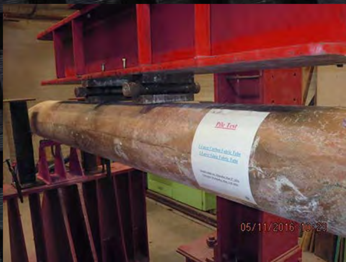
PVC pipe shells were removed to test the true standalone loading capacity.
