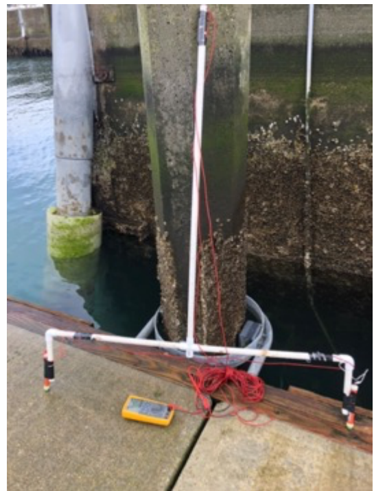
Figure 1: Voltage Gradient Test Locations and Test Apparatus
